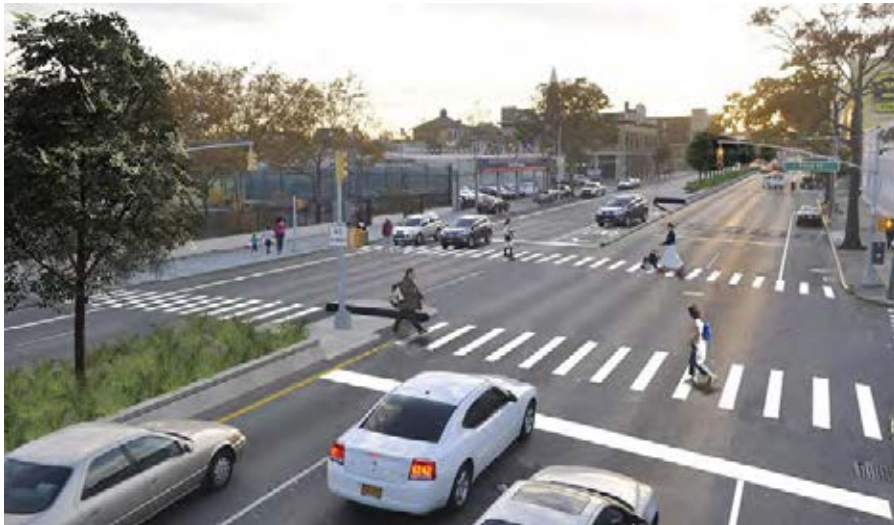
Figure 22 – Example of a median refuge island at a signalized intersection. Source: visionzerostreets.org
